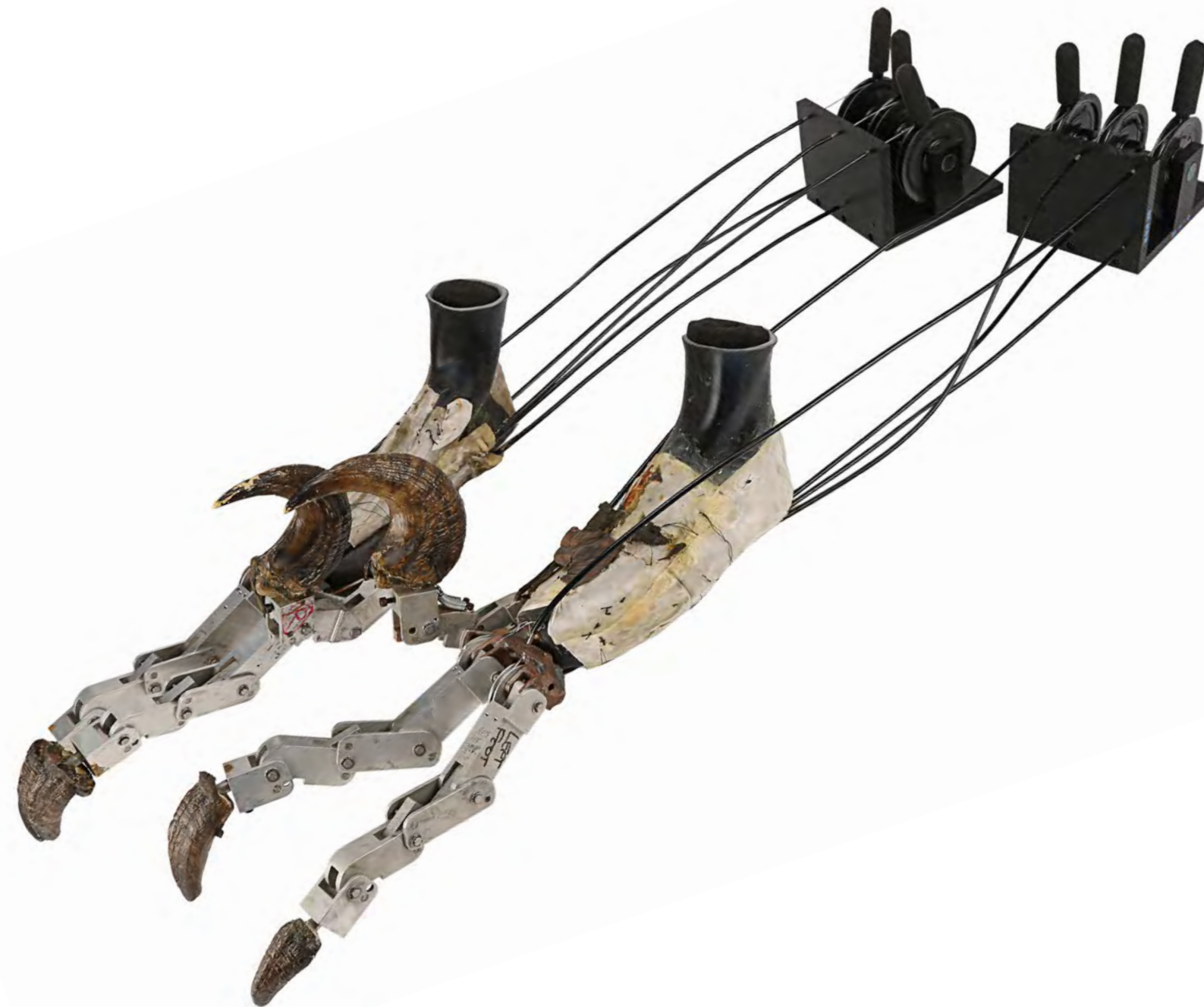
424. Cable-Controlled Velociraptor Puppet Feet With Claws
