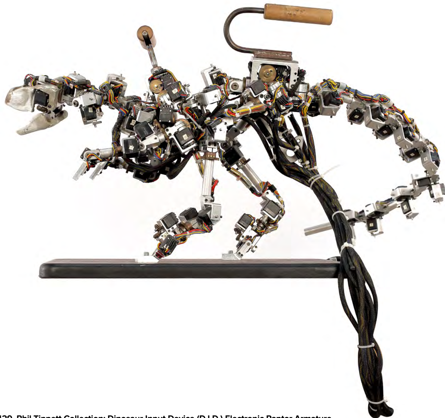
429. Phil Tippett Collection: Dinosaur Input Device (D.I.D.) Electronic Raptor Armature
