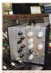
Three Olympic '65 modules, From left: an original EQ module from the 'reduction stud (later Studio Three), an input module from to Studio One desk at Olympic Barnes, origina installed in 1966, and a new recreation of the same mic amp, complete with germanium transistors and a balanced output stage to interface with modern-day equipment.
