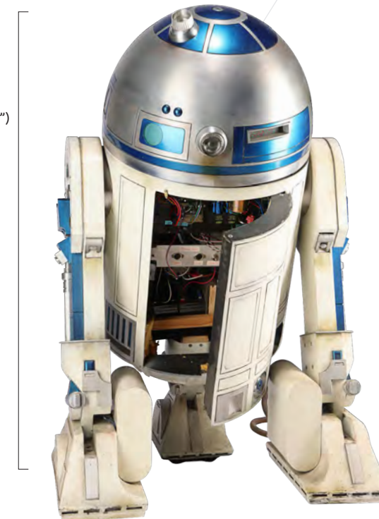
Dome and body are made of aluminium
