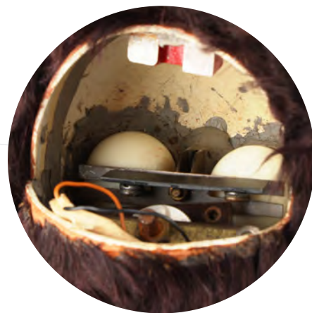
Interior head detail reveals the solenoid and eye mechanism
