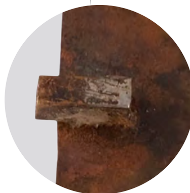
Two small square pieces of metal have been welded onto the back, allowing the plate to be rigged on a SFX rig to achieve the special spinning effect
