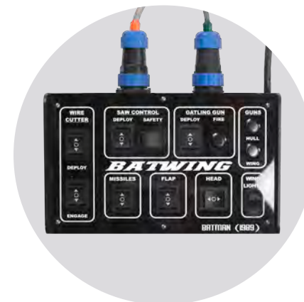
Updated control box powers servos and linear actuators for the model's mechanical functions
