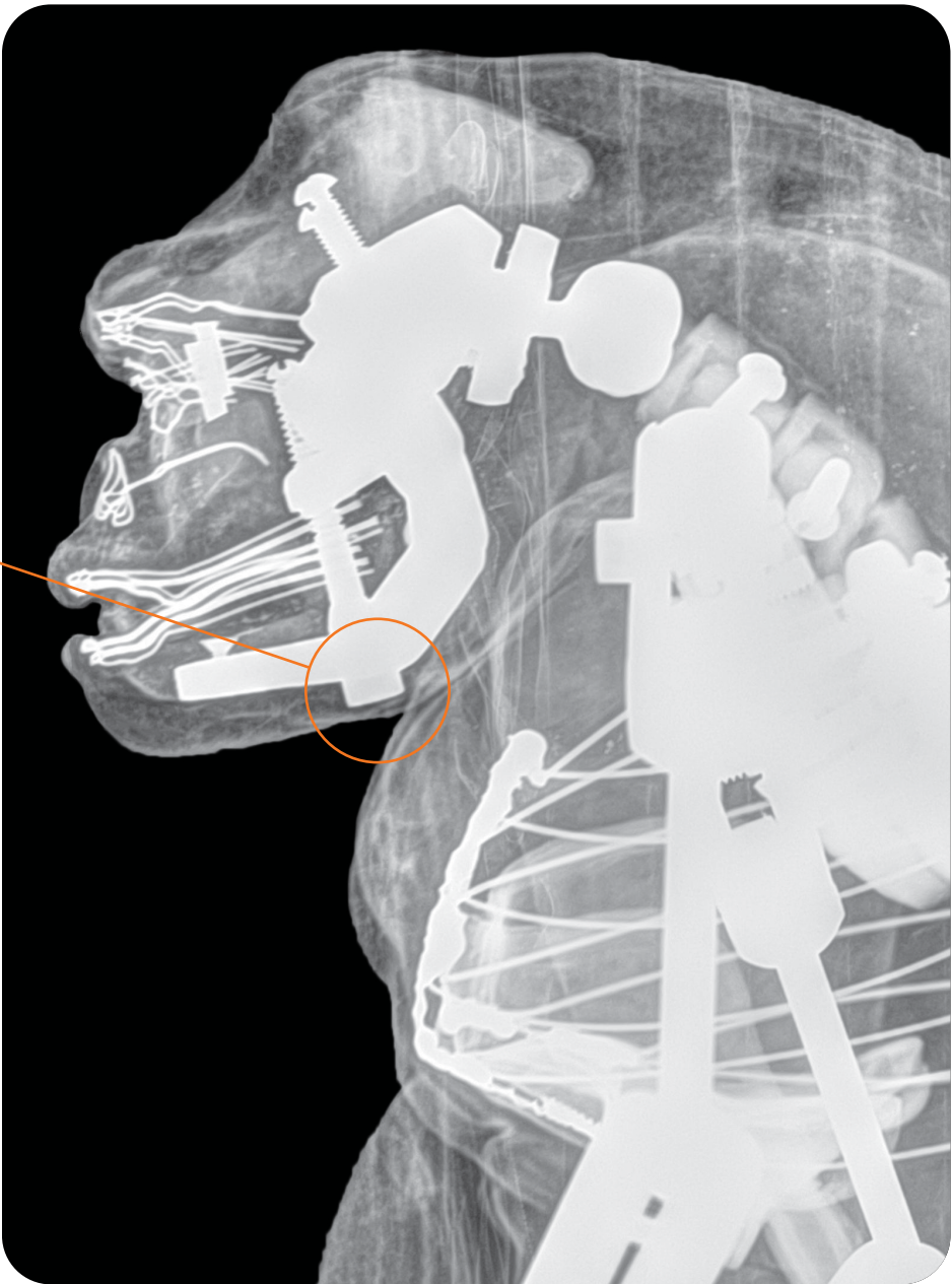
The fine lines visible in the face are thin pieces of wire embedded in the skin so that the lips, nose and eyebrows can hold their position while being animated.
